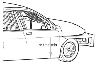
heads of those pins/bolts must be protected. Wheel guards must be in place at all times and must cover the top of the tyre to wheel level, to include at least 75mm of the tyre.
