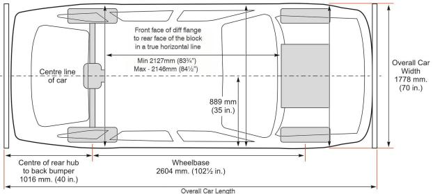
Overall Car Length Min 4318mm (170") to Max 4369mm (172")
