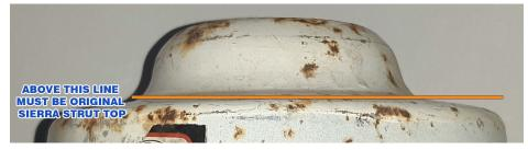
mounted within 5mm of original position checked by two methods; firstly from carburettor and secondly from front face of pulleys. A tolerance of 50mm is permitted on the passenger side strut top taken from the original centre point, forward or back. You are permitted to move the strut top in towards the engine to achieve camber.
