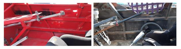
• Where the driver's side doors (front and rear) meet the lower window aperture, this must be backed by RHS or equivalent tube, a minimum of 25mm x 25mm, 3mm thick. This should be supported from either/both the roll cage or top rail. Additionally, if the roll cage is not supporting the B pillar (and is
